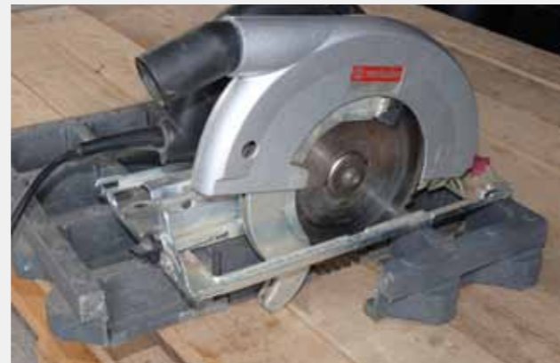
Suitable devices according to the cutting direction: straight: Circular saw with a tungsten carbide tipped saw blade round: Saber jig saw (take the element height into account)
